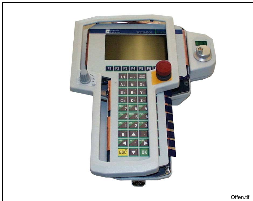
Fig. 4-1: An open BTC06 with a view of the slide-in strips
