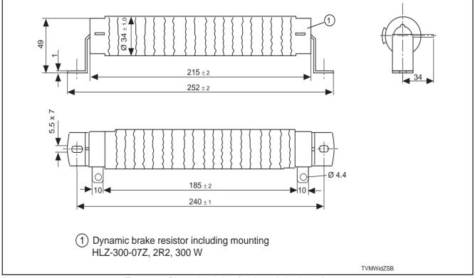
Figure 7.8: Dimensional data for dynamic brake resistor
