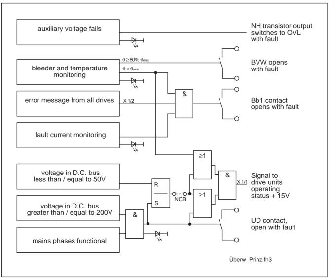
Figure 5.3: Diagram of interfaces for monitoring and diagnostics systems
