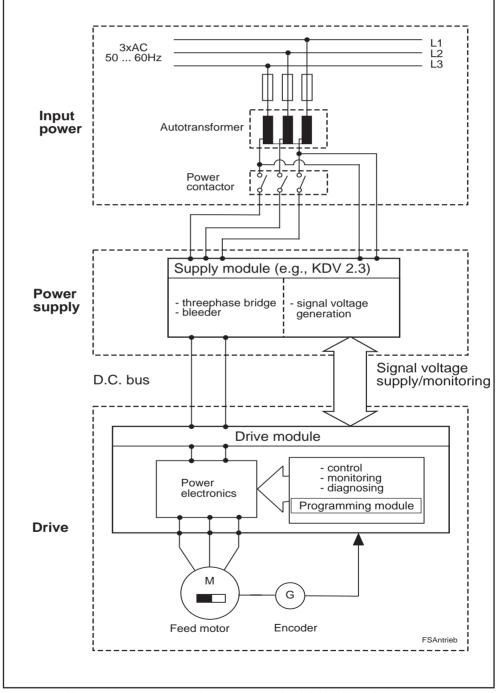
Figure 1.1: The KDV 2.3 supply module as a part of INDRAMAT's AC drive system
