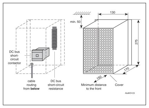
Fig. 4.3: Suitable covers and unit arrangements for the DC bus short-circuit
