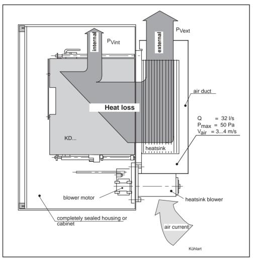
Figure 3.14: A break down of the heat losses
