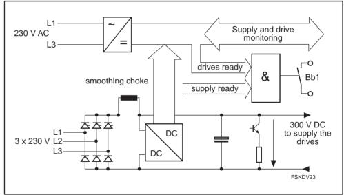
Figure 1.2: The design of the KDV 2.3 supply module
