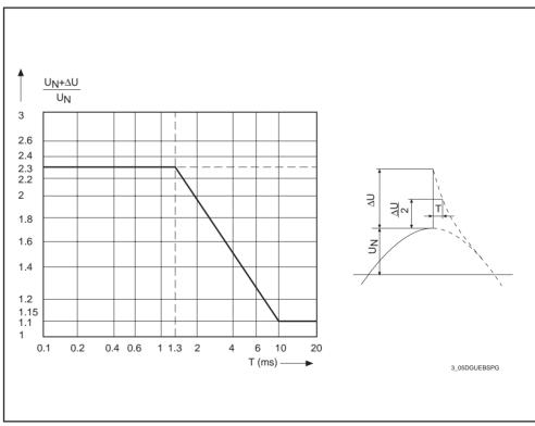
Figure 3.6: Permissible non-periodic overvoltages per VDE 0160
