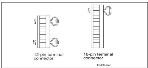
Figure 3.10: Terminal connector for the wire-ribbon connection
