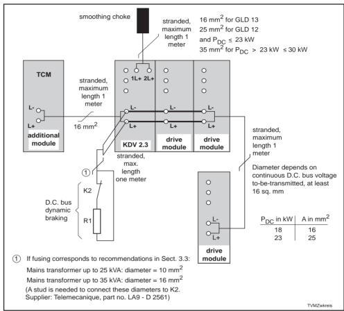
Figure 3.7: DC bus wiring
