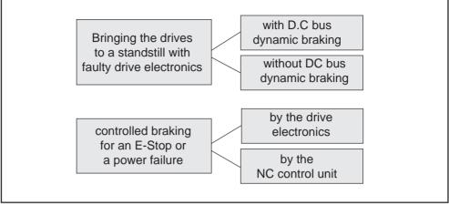
Figure 4.1: Differentiating features of the power circuits
