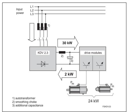
Figure 2.1: Power range of a KDV 2.3 supply module
