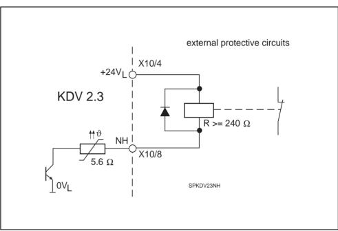
Figure 5.2: Protective circuit of the NH transistor output
