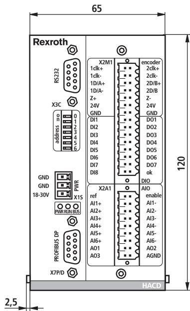
Installation on top hat rail TH 35-7,5 or TH 35-15 according to EN 60715
