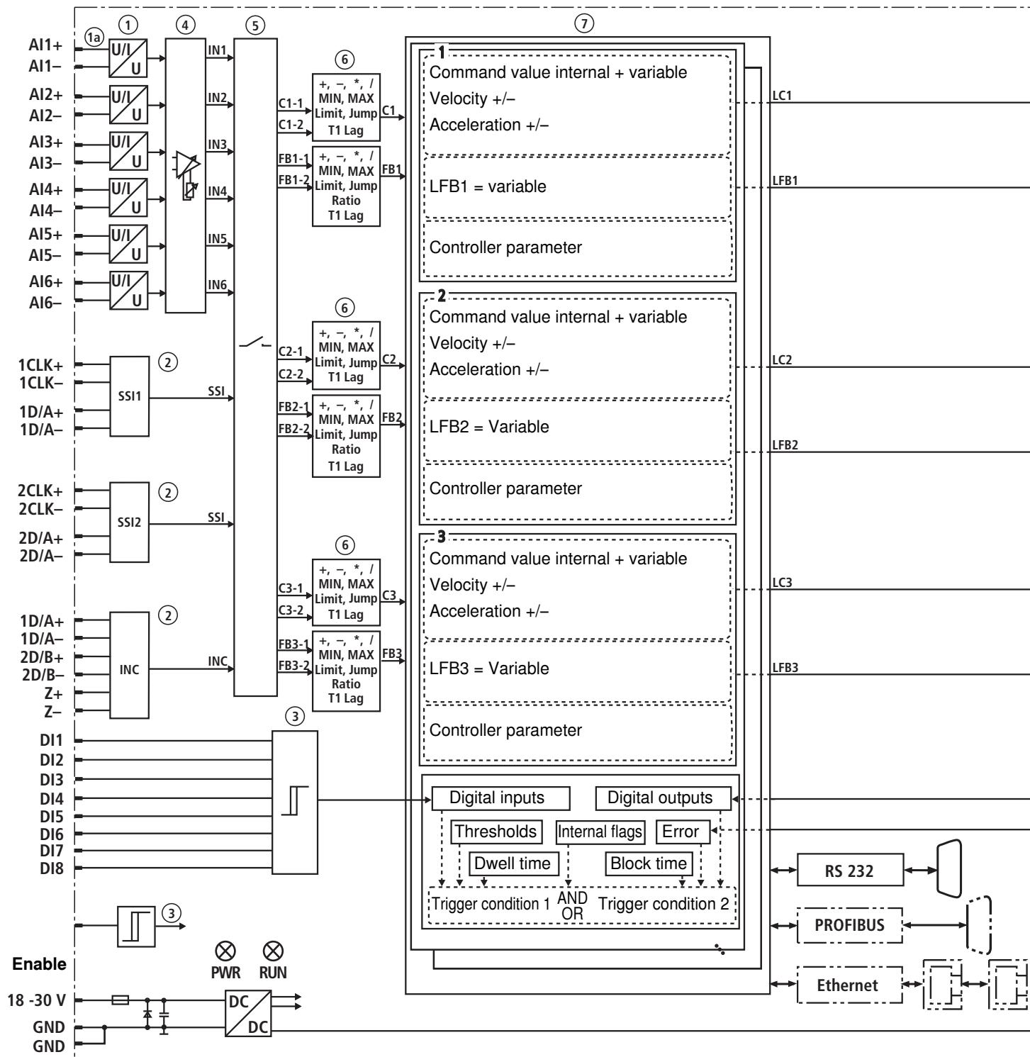
1 Analog inputs voltage or current
