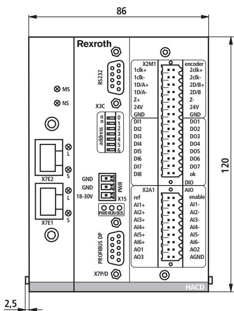
Installation on top hat rail TH 35-7,5 or TH 35-15 according to EN 60715
