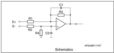
R1: 10k R2: 10k R3: 20k R4: 20k C1: no data C2: no data Fig. 4-85: Input circuit
