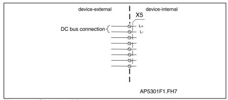
Fig. 6-39: Connection DC bus
