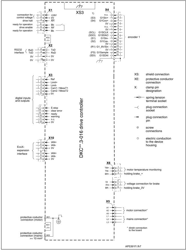
Fig. 5-21: Total connection diagram for DKC\*\*.3-016
