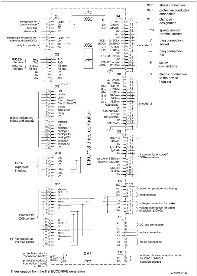
Fig. 4-47: Total connection diagram for DKC\*\*.3
