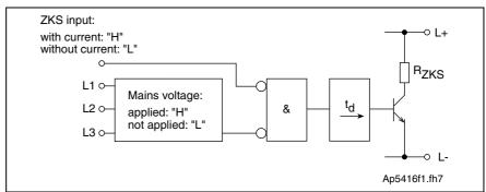
Fig. 4-146: Block diagram interlock ZKS/Mains
