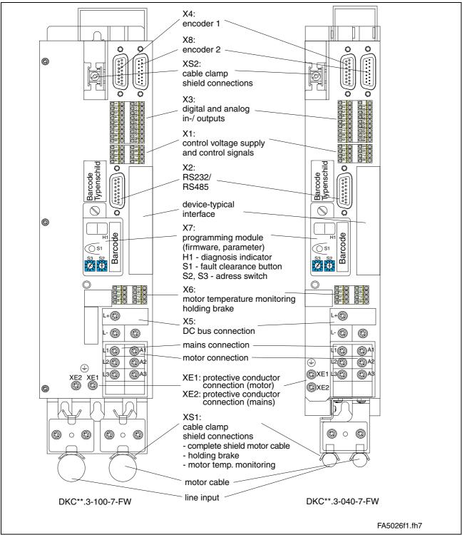
Fig. 4-43: Front view DKC\*\*.3-040-7-FW and DKC\*\*.3-100-7-FW with Connectors
