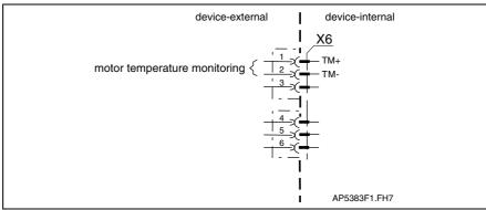
Fig. 5-62: Motor temperature monitoring
