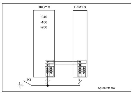
Fig. 6-10: DC bus and mains connection
