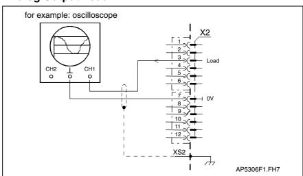
Fig. 6-26: Output load
