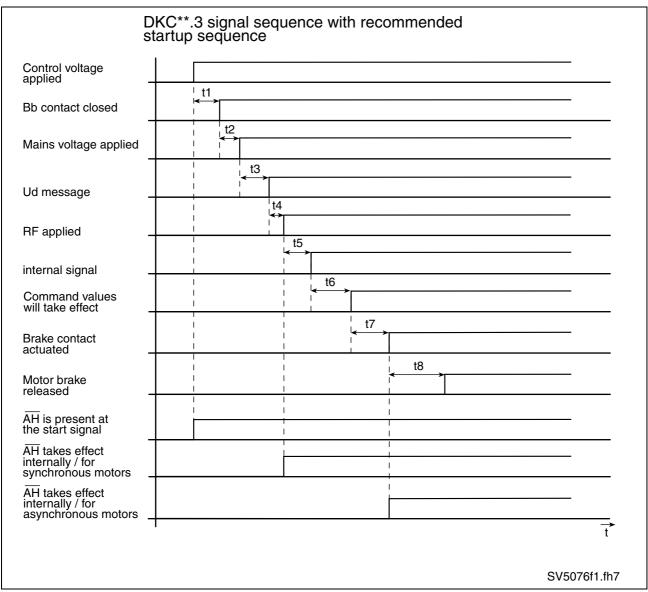
Fig. 16-38: Recommended switching on sequence
