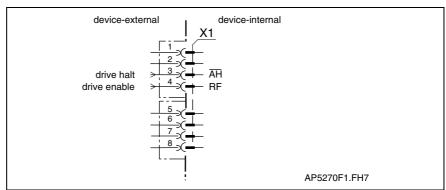
Fig. 4-53: Connections for drive halt and drive enable
