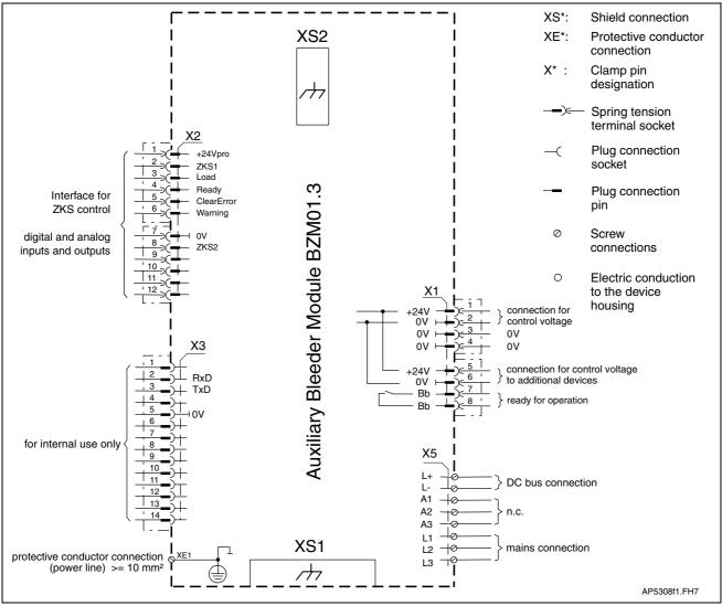
Fig. 6-9: Terminal diagram - BZM01.3
