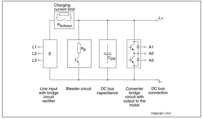
Fig. 4-8: Block diagram of the DKC\*\*.3-040-7-FW power section
