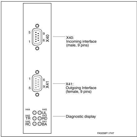
Fig. 4-193: View of command communication interface
