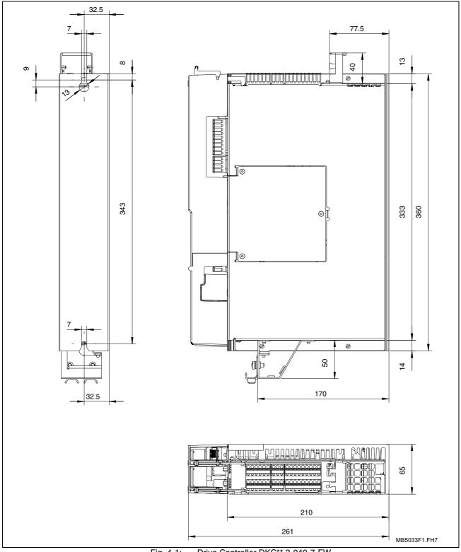
Fig. 4-1: Drive Controller DKC\*\*.3-040-7-FW
