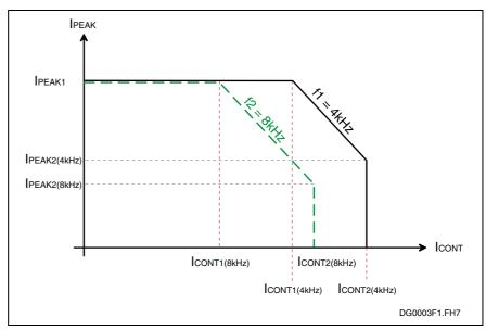
Fig. 5-8: Output current characteristic curves for servo applications
