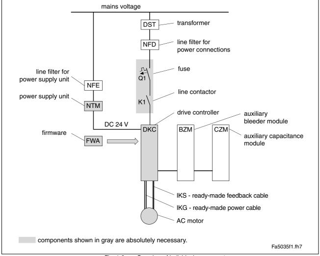
Fig. 1-2: Overview of individual components
