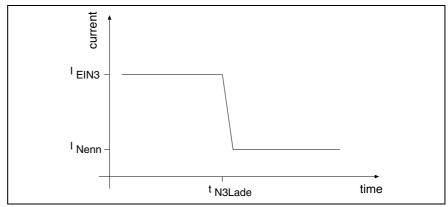
Fig. 4-13: Example of charging current inrush of control voltage
