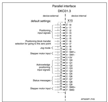
Fig. 4-162: Parallel interface for DKC01.3
