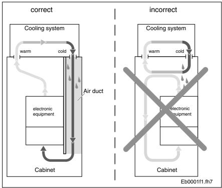
Fig. 12-19: Arranging cooling unit on cabinet
