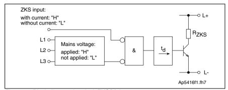
Fig. 6-25: Block diagram interlock ZKS/Mains
