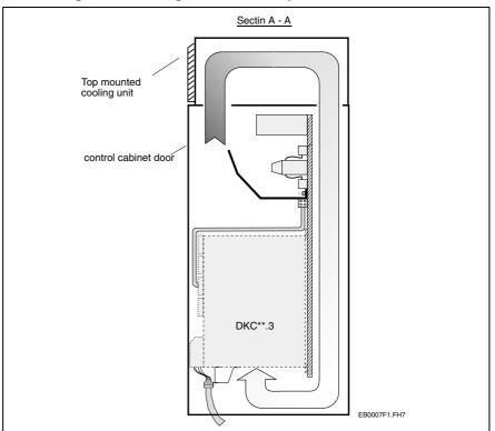
Fig. 16-16: Mounting the cooling unit onto top
