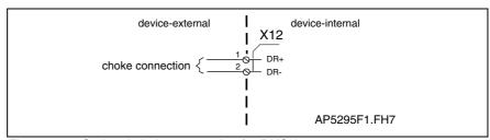
Fig. 4-154: Optional choke connection for DKC\*\*.3-200-7
