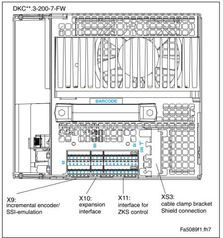
Fig. 4-46: Connections on top of unit for DKC\*\*.3-200-7-FW
