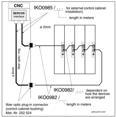
Fig. 4-180: Selecting standard fiber optic cables
